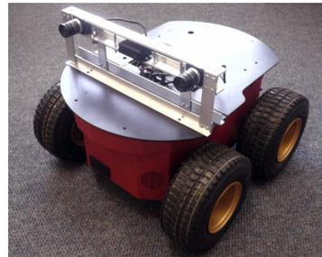
Fig. 2. Our Pioneer 3-AT robot, with two Point Grey Firefly MV cameras in a stereo configuration and an external synchronisation unit, used for capturing datasets.
