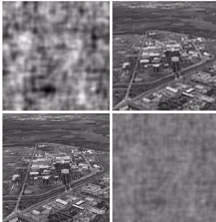
FIGURE 5.27 Restoring Fig. 5.25(b) with Eq. (5.7-1). (a) Result of using the full filter. (b) Result with H cut off outside a radius of 40; (c) outside a radius of 70; and (d) outside a radius of 85.
