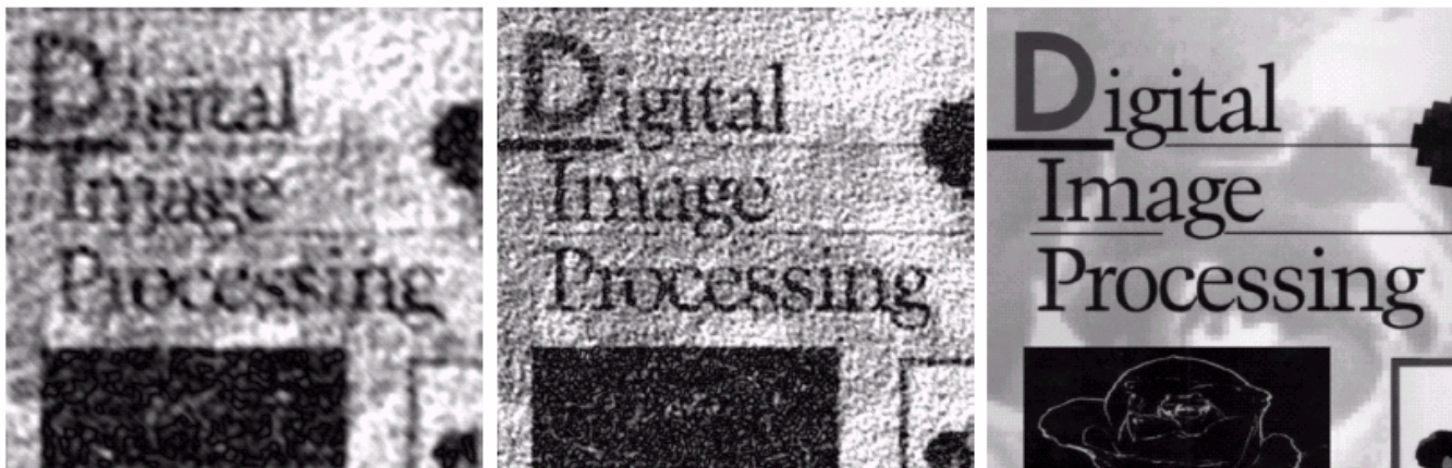
FIGURE 5.30 Results of constrained least squares filtering. Compare (a), (b), and (c) with the Wiener filtering results in Figs. 5.29(c), (f), and (i), respectively.
