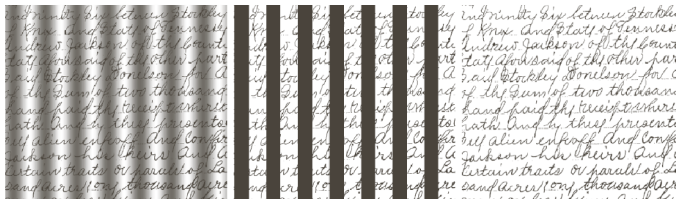
FIGURE 10.50 (a) Text image corrupted by sinusoidal shading. (b) Result of global thresholding using Otsu's method. (c) Result of local thresholding using moving averages.
