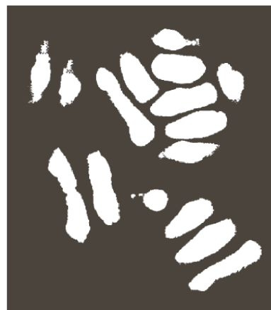
FIGURE 10.44 Image in Fig. 10.43(a) segmented using the same procedure as explained in Figs. 10.43(d)–(f), but using a lower value to threshold the absolute Laplacian image.
