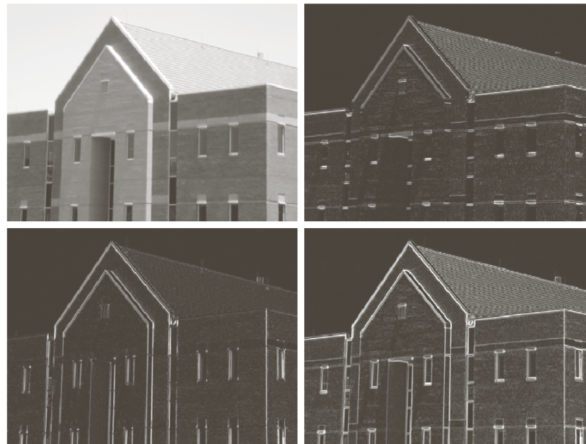
FIGURE 10.18 Same sequence as in Fig. 10.16, but with the original image smoothed using a 5 \times 5 averaging filter prior to edge detection.
