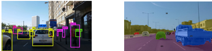
Fig. 3. Faster R-CNN object detection [16] or Panoptic FCN image segmentation [17] can guide attention regions. The former produces bounding boxes around objects (left), and the latter a pixel-level mask around objects and salient image regions (right).
