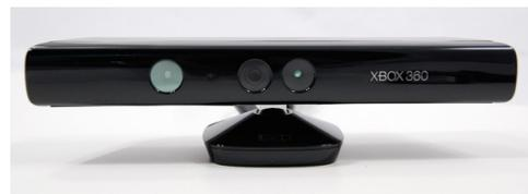
Fig. 1. The Microsoft Kinect sensor with IR projector, RGB camera and IR camera visible from left to right.
