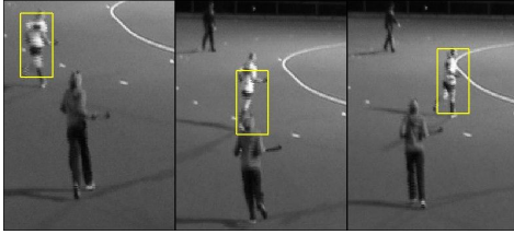
Figure 6: Before, during and after a partial occlusion. The tracker successfully follows the partially occluded player.
