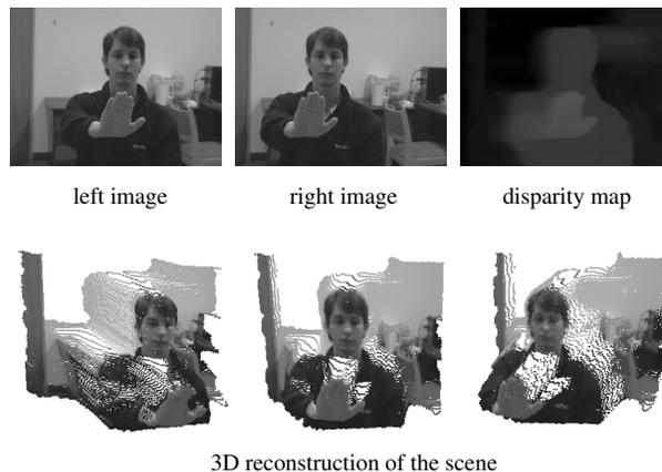
Figure 1: An example of a dense 3D reconstruction from a stereo pair of images.
