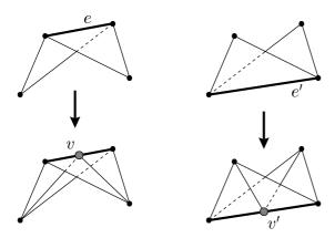
Figure 3: Adding points to the triangulation.
