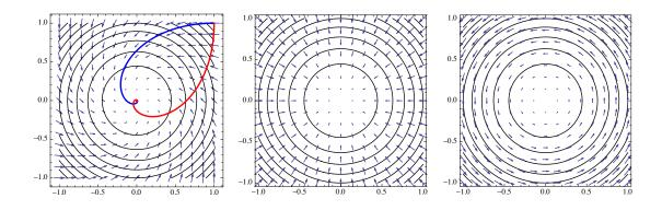
Figure 4: Linear transversal system. Left: Natural decay path (blue) and instanton (red) superimposed on the vector plot of total force. Middle: Vector plot of the dissipative force. Right: Vector plot of the stream force. The black lines in the plots are equi-potentials of the quasi-potential V(x, y).
